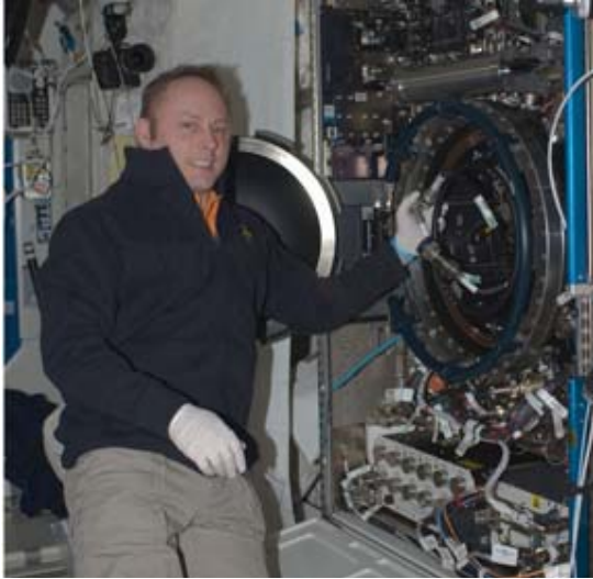
Astronaut Mike Fincke completing install of the CIR/MDCA insert prior to CIR activation in January 2009.
