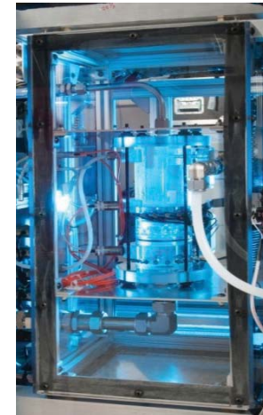
The TPFSE test sections, DYNAFLOW (left) and CWRU (right), with containment for integration in a test rig for testing
