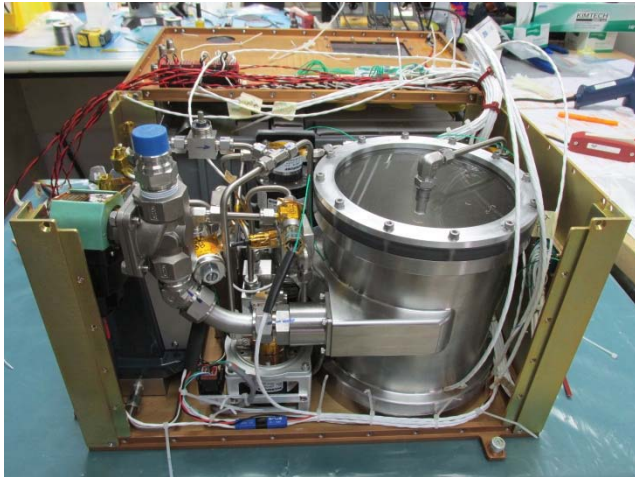
Pumped Separator for PBRE
