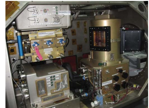
ZBOT Engineering Model in the MSG Work Volume Mockup
