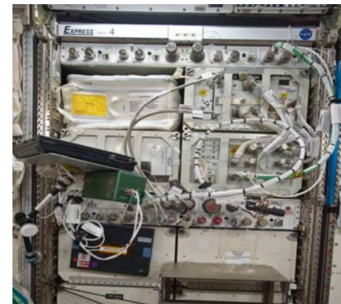
DECLIC installed in an EXPRESS Rack on board ISS
