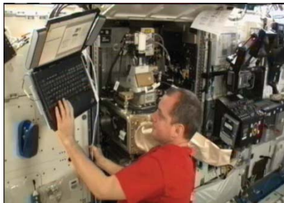
Astronaut T. J. Creamer installing the first CVB Module on March 20, 2010.
