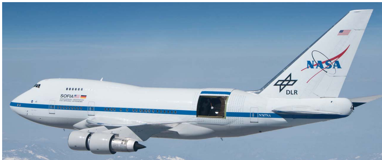
Figure 1. Aircraft with large cutout.
