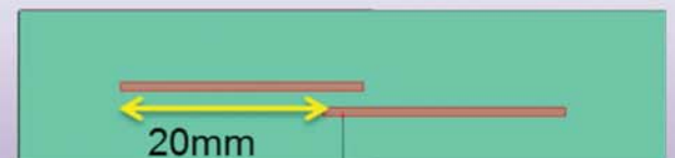
Case 3: discontinuous wires, offset by 20 mm
