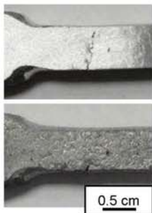
Cast overload sample pre- and post-healing
