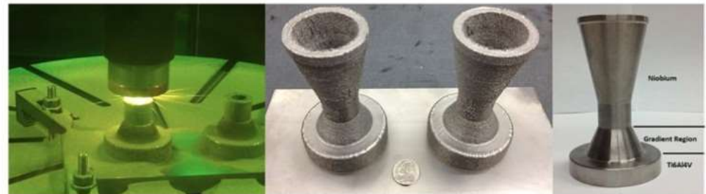
Prototype titanium to niobium gradient rocket nozzle
