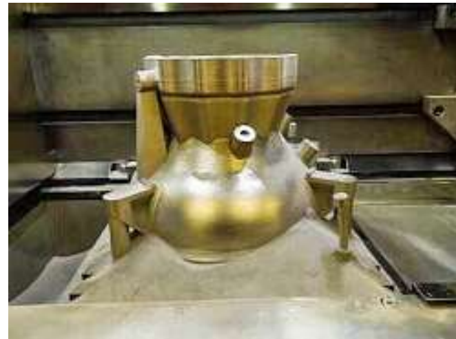
SpaceX SuperDraco combustion chamber for Dragon V2 made from Inconel using the DMLS process
