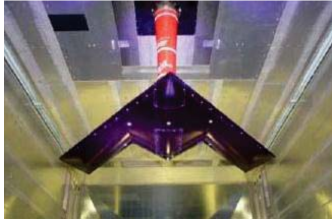
Figure 8. SACCON configuration in the Low-Speed Wind Tunnel, Braunschweig Germany (DNW-NWB). \Lambda_{le} = 53^\circ .
