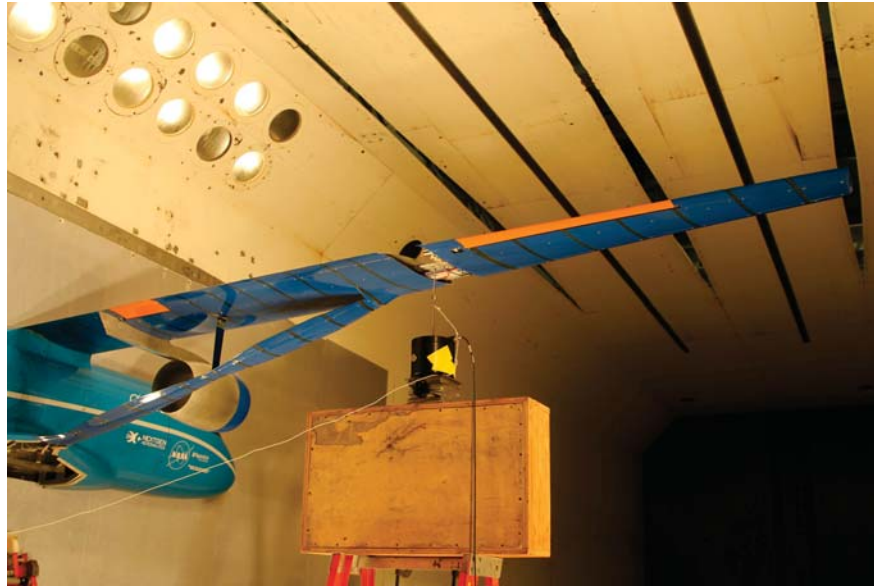
Figure 7. GVT shaker set-up of the TBW wind-tunnel model in the TDT.
