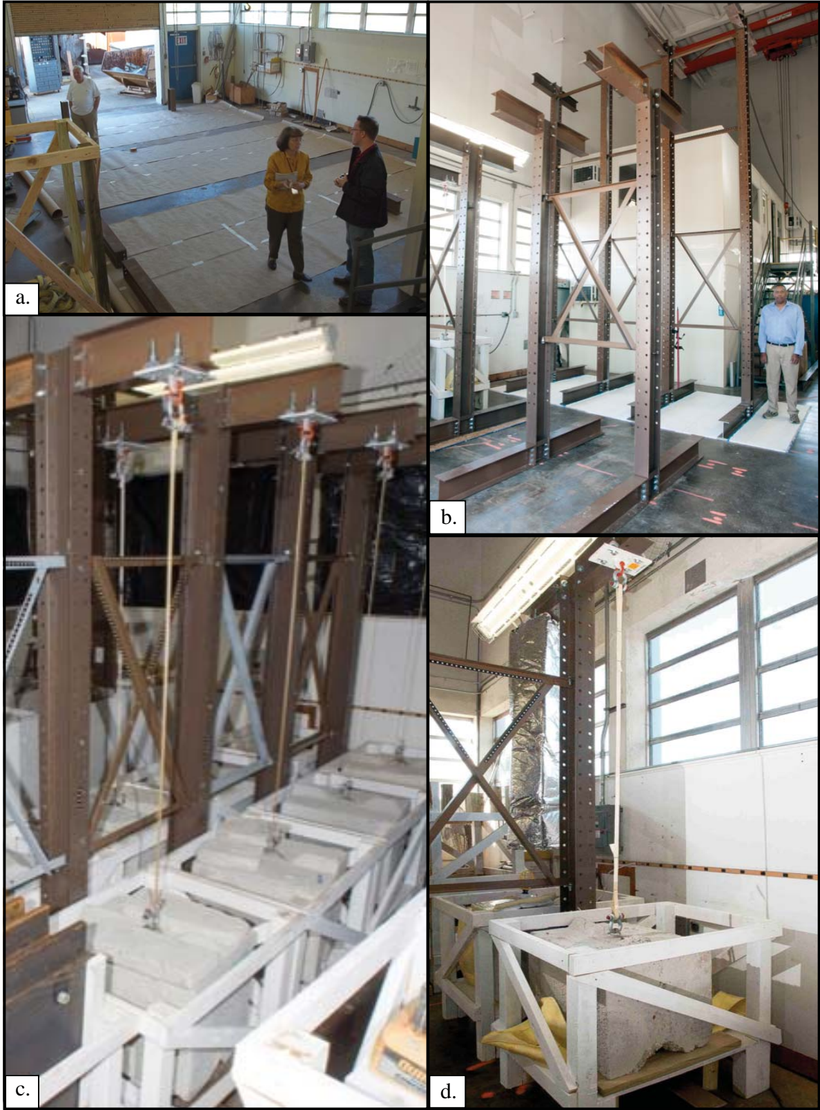
Figure 8. Test facility build: a.) empty facility, b.) two rows of double cantilevered I-beam structure, c.) row one of Kevlar & Vectran creep tests, d.) typical creep test.
