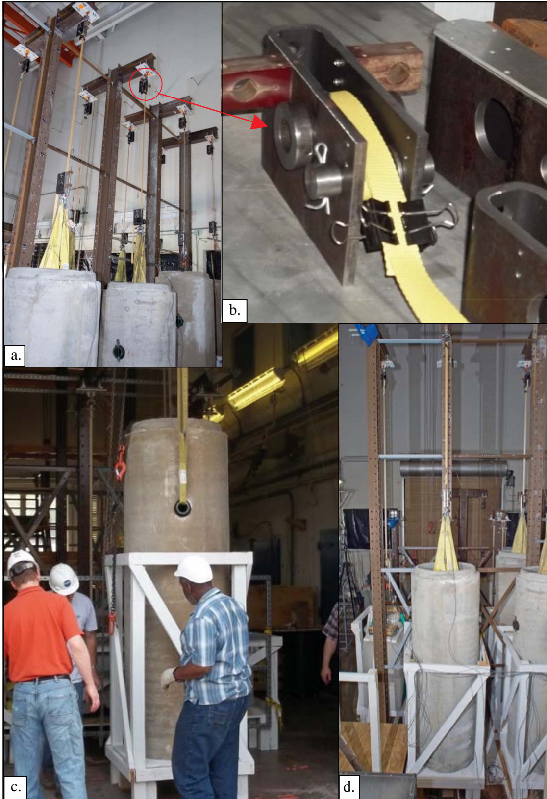
Figure 9. Hardware for second row of creep tests; a.) four Kevlar tests, b.) custom restraint fixture with webbing, c.) concrete culvert weight, d.) typical creep test.
