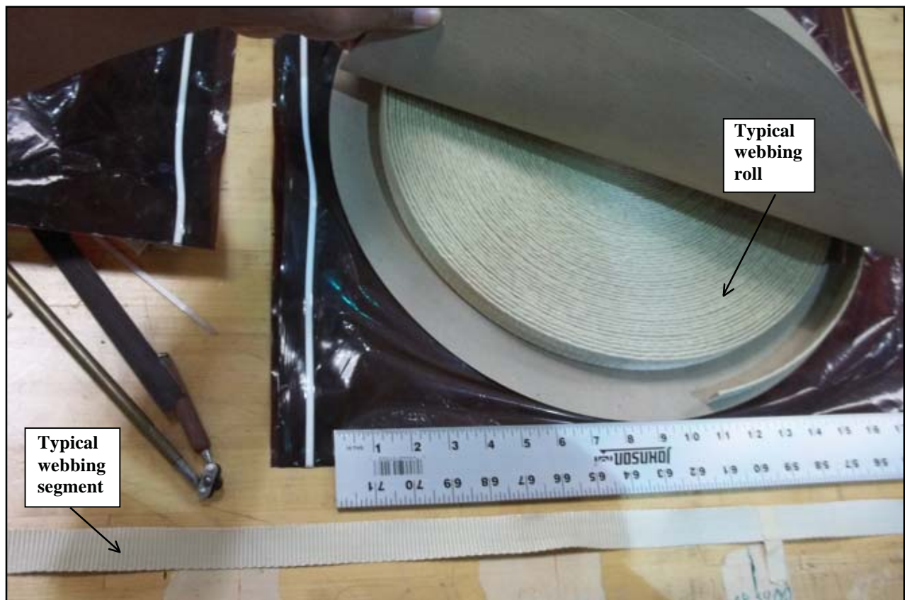
Figure 7. Typical roll and segment of Vectran webbing.
