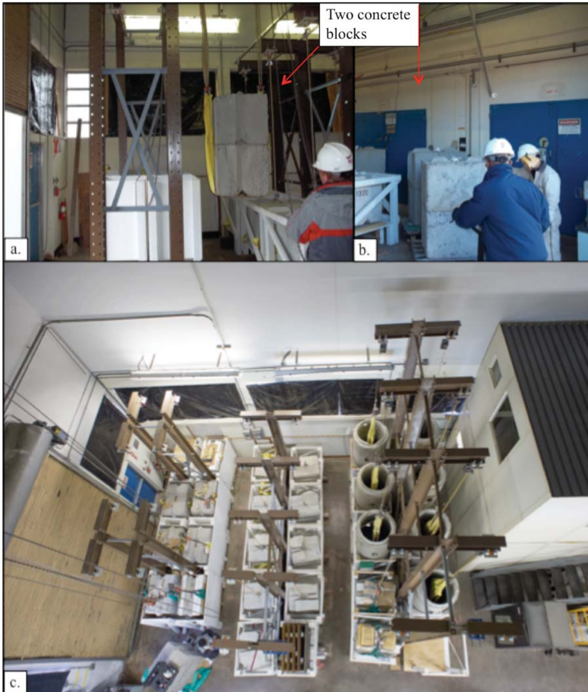
Figure 10. Hardware for third row of creep tests and top view of test site; a.) two concrete block weights being lifted into containment structure, b.) positioning of two concrete blocks with pallet jack, c.) top view of fully populated and operational creep test facility.
