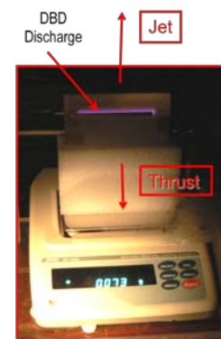
Figure 3. Setup of an actuator on an analytical balance
