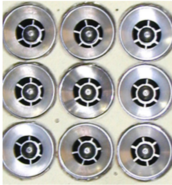
Figure 3: Baseline 9-point SV-LDI design. From R. Tacina et al. 1
