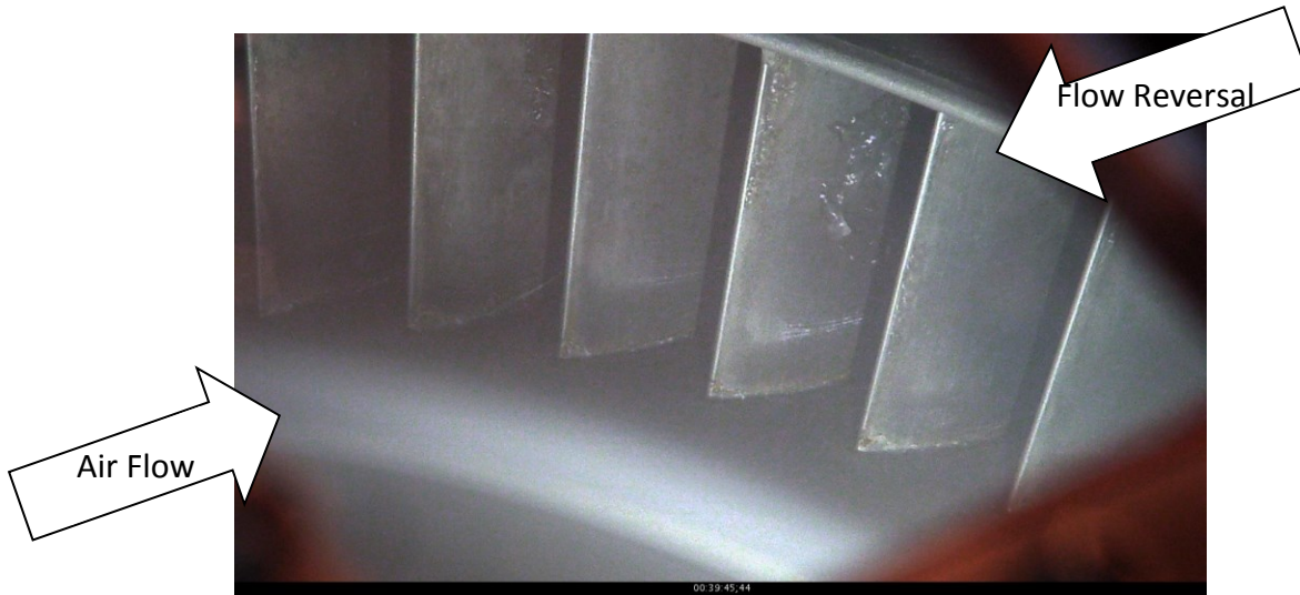
Figure 16: Image capture from video taken during the PSL engine testing of the IGV showing water flowing upstream on the IGV surface beyond Escort scan 180. This is evidence of air flow reversal and corroborates the results of the computational flow analysis, indicating a stalled LPC.
