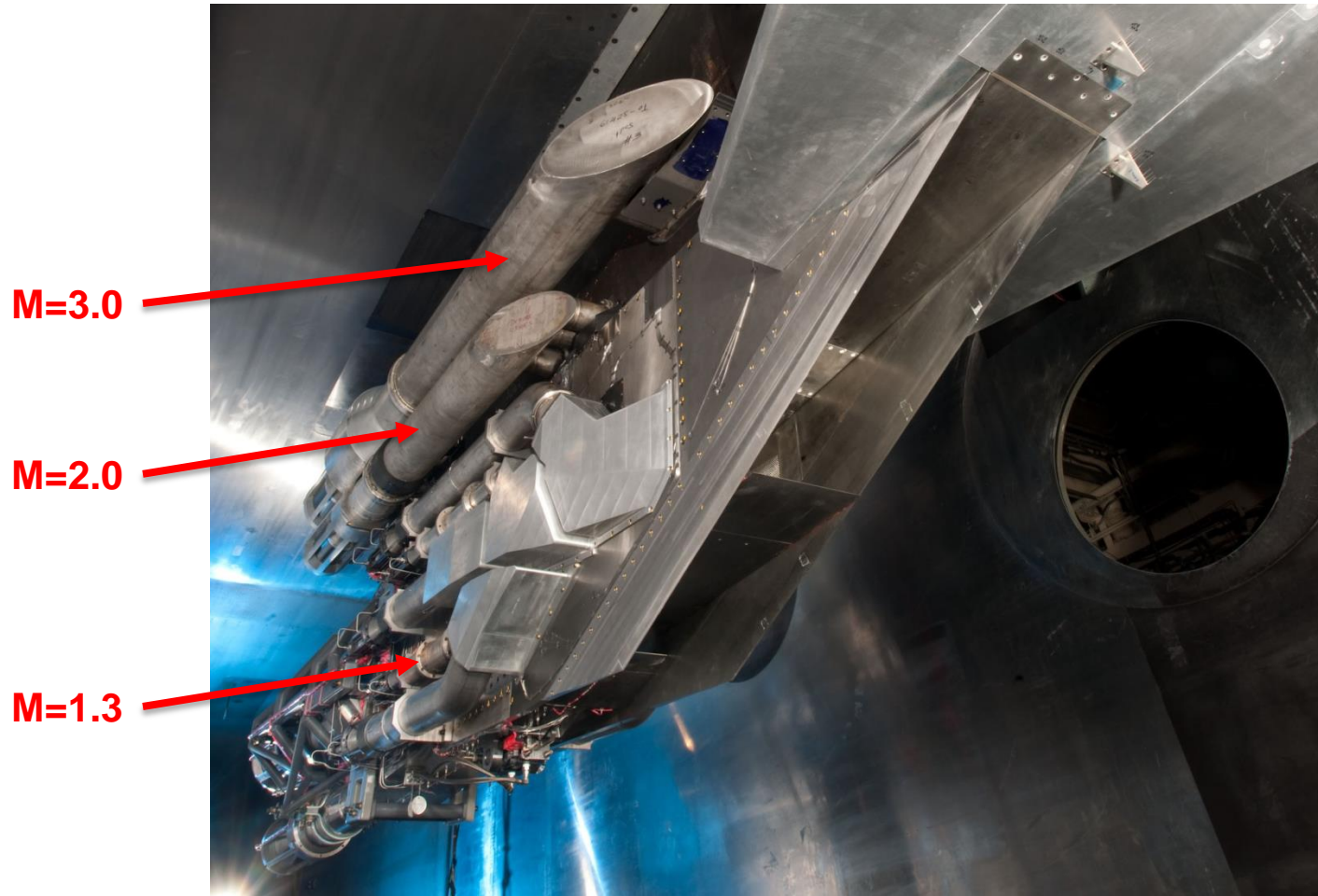
LIMX Model – Uncooled bleed ductwork size as a function local Mach number
