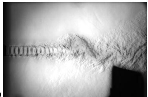
Fig. 12 Schlieren pictures of flowfield for the OL case at three different M_j ; x_{TE}=8.5'' , z=-1.2'' . (a) M_j=0.67 , (b) M_j=0.96 and (c) M_j=1.03 .
