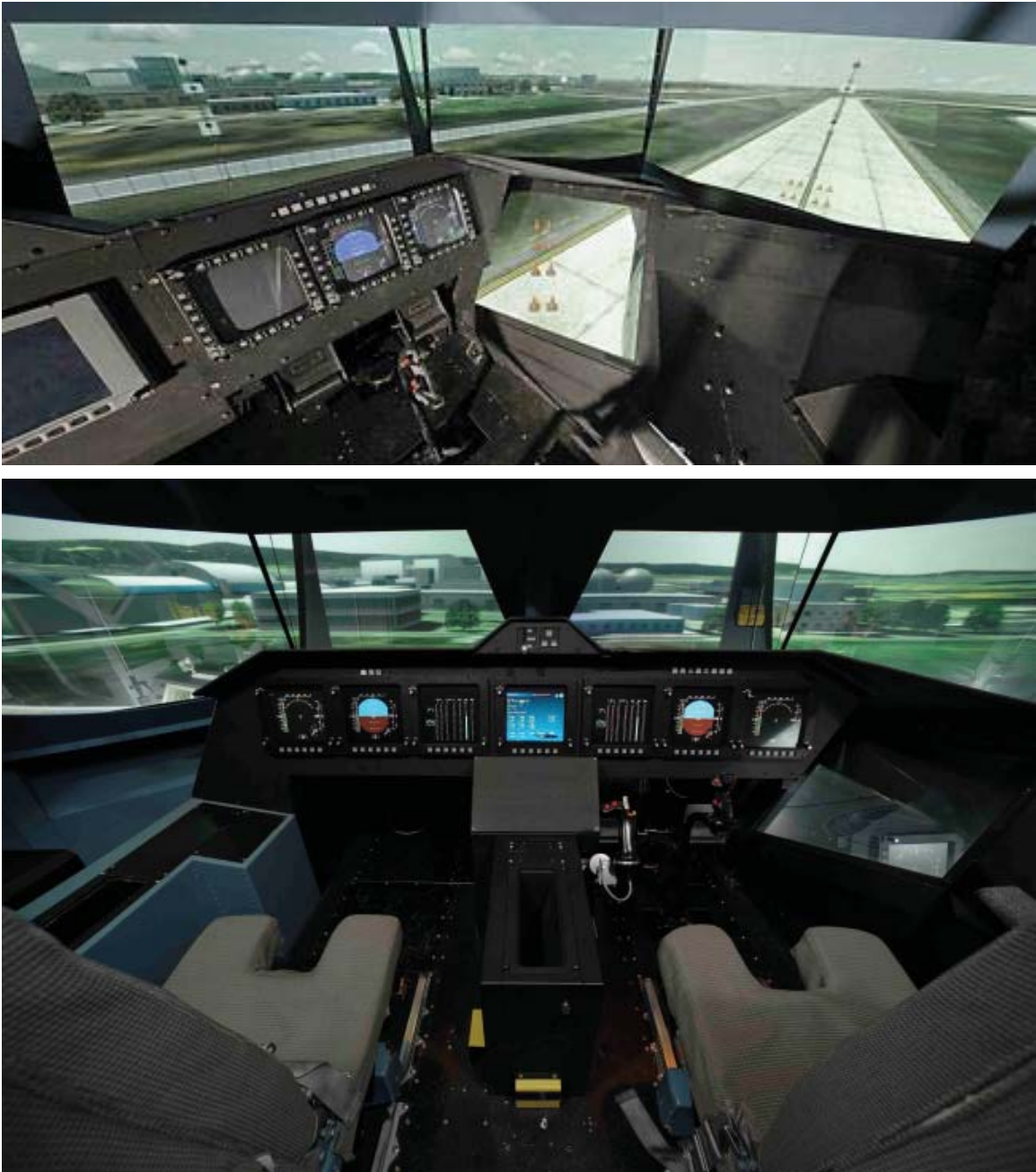
Figure 17. VMS two-seat transport cab overview.
