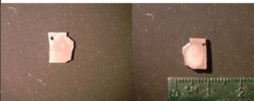
Figure 4: CMNH-Pyr-R3u 15h with a scale on the B side. The lack for luster for this sample as compared to the before sample is most evident due to alteration to pyrrhotite. There are also some cracks and fissures in the sample best evidenced by the cracks in the upper left side of the side A sample.
