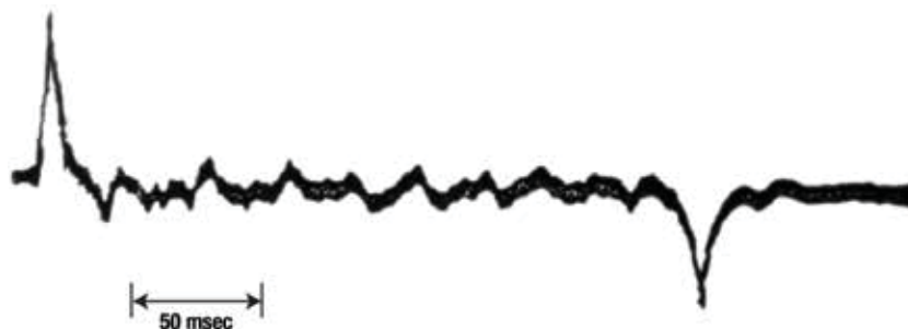
Figure 9.146. Experimental pressure waveform from straight linear charge of uniform explosive linear density, length 60 in. (ref. 9.88).
