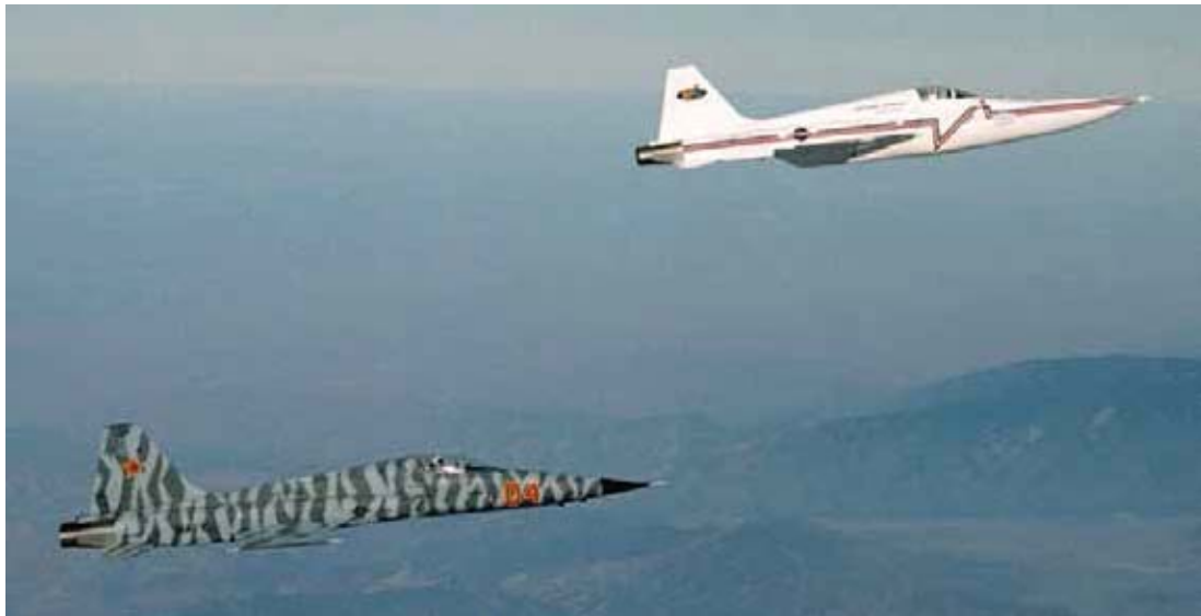
Figure 4.19. The Shaped Sonic Boom Demonstrator (SSBD) aircraft (top) performs a research flight while a U.S. Navy F-5E flies chase.
