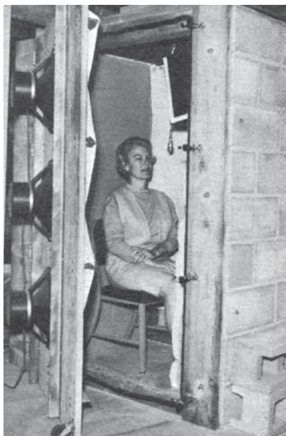
Figure 9.110. Lockheed Sonic Boom Simulation Chamber – note hinged wall access (ref. 9.62).
