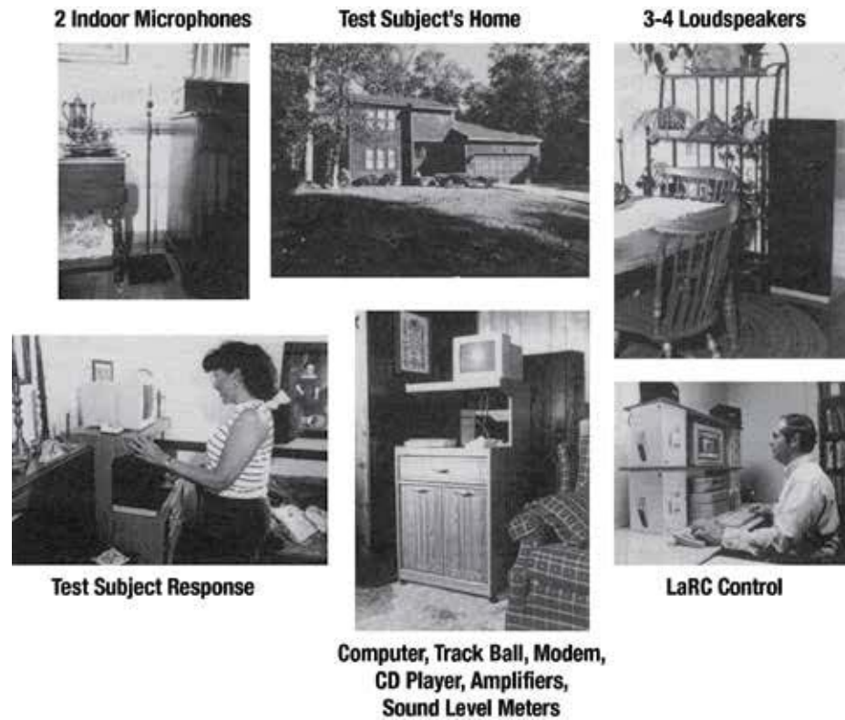
Figure 9.127. In-home noise generation/response system (ref. 9.76).
