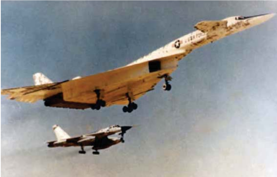
Figure 4.8. The North American XB-70A Valkyrie, escorted by a B-58 Hustler chase aircraft, making a landing approach at EAFB. The XB-70, in normal flight configuration, is showing paint job wear resulting from the rigors of the high-speed flight-test regime.
