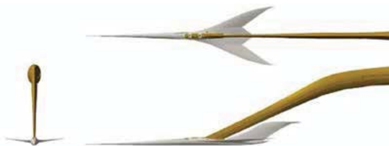
(a) Three-view drawing of wing-body-vertical low-boom aircraft concept with a blade mount.
