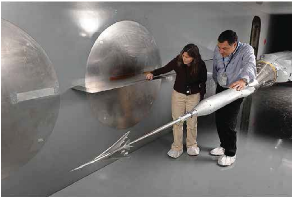
Figure 9.24. RF 1.0 pressure rail mounted on the aft window blank at the NASA ARC 9 - by 7-foot Supersonic Wind Tunnel (ref. 9.16).
