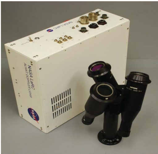
Figure 4. Prototype Doppler lidar system consisting of an electronic chassis and an optical head
