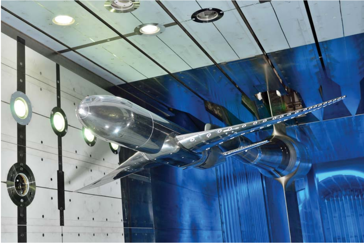
Figure 9. Photo of the Common Research Model in the European Transonic Wind Tunnel.
