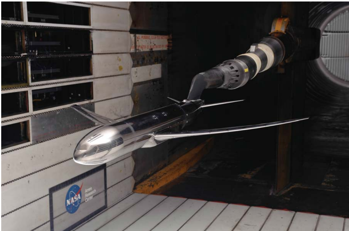
Figure 8. Photo of the Common Research Model in the Ames 11-ft Wind Tunnel.
