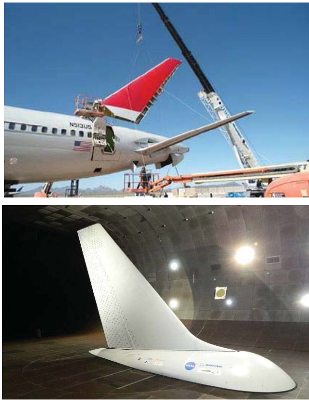
Figure 4. Boeing 757 vertical tail being removed at Evergreen Air Center (top) and the tail model installed on top of a blister fairing in the NFAC 40x80 wind tunnel (bottom).
