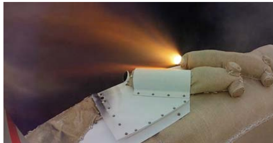
Figure 7. Image from cameras on-board SFDT-1 showing spin motor plume interacting with test vehicle surface.
