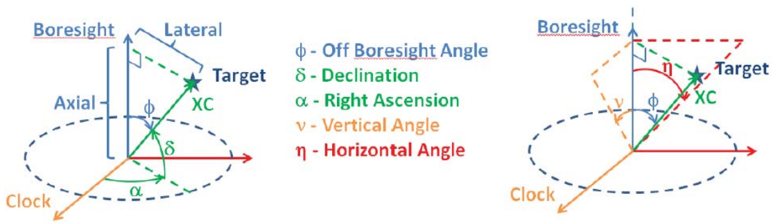
Figure 2. Graphical Description of the Antenna Subsystem 2
