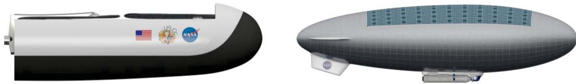
Figure 3. Notional entry vehicle aeroshell (left) and airship (right) designs. Images are not to relative scale.
