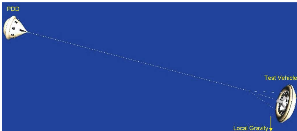
Figure 4: Visualization of PDD Trailing Behind LDS Test Vehicle Based on POST2 Multi-Body Simulation Output
