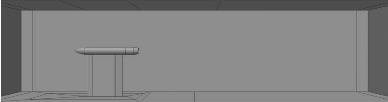
Figure 5. Jet modeled in GRC 1x1 SWT test section.
