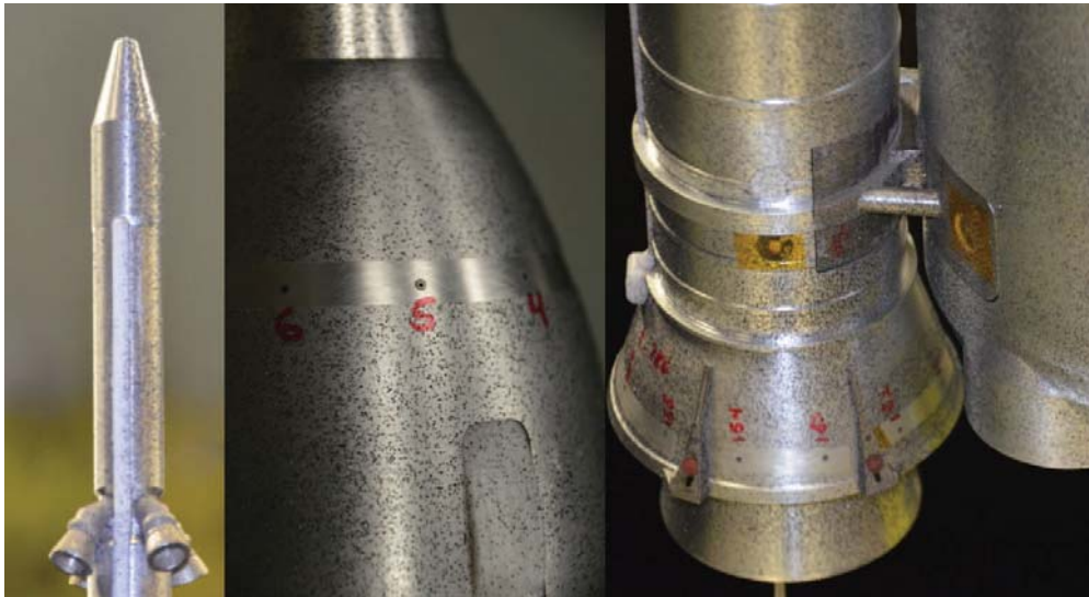
Figure 3. Close-up pictures of various surfaces on the SLS wind tunnel model showing the uniformly sprinkled #80-grit for boundary layer tripping.
