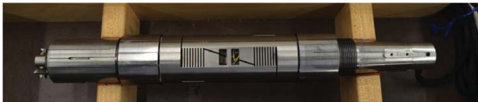
Figure 12. NASA Langley Strain Gauge Balance 756; front balance expander is on the left side, and sting taper on the right.
