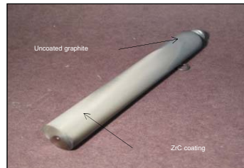
Above: Test Piece highlighting ZrC Coating Right: Coating primarily on external surface
