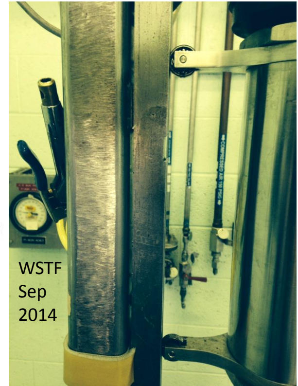
Spider plummet bearings are in the guide tract.
