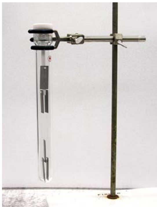
Figure 2. Metal coupons suspended in a high-pressure-rated glass tube.
