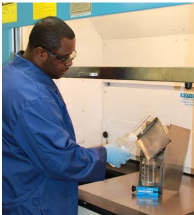
Figure 5. Configuration to flush a test panel for the NVR removal efficiency test.
