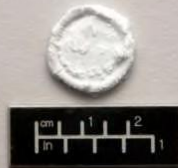
WSTF NO. 14-46299 Solvokane Pressure Screen LOX NASA-STD-6001.B Test 13BP Post Purge
