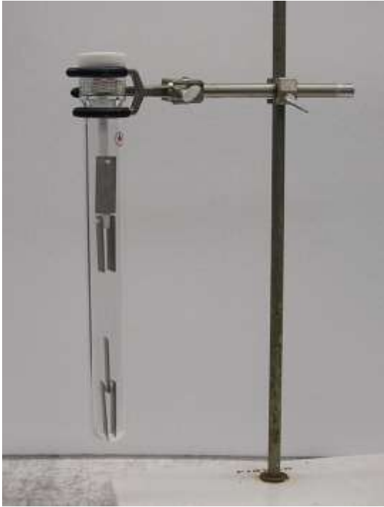
Coupon set in HP Glass Tube. Heavy Wall Glass Tube Rated at 150 psig, Tube Vol. 210 ml.
