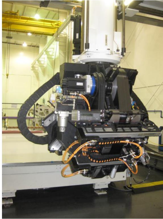
Figure 1. MAG-IAS Low Rail Charger Tape Placement Head
