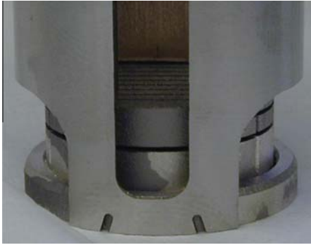
Fig. 6. Tungsten magnetoresistive heat switch which is sliced into a meander path (center of picture). Above the switch is a copper bus bar and below the switch is a mounting surface to an ADR stage.
