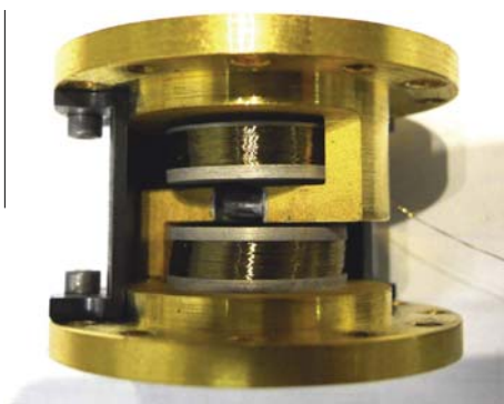
Fig. 5. Superconducting heat switch used in a CADR for temperatures below 0.35 K. The Helmholtz coil is stacked around a lead rod in the center of the picture. Gold-plated copper carries the heat between the top and bottom flanges. Vespel™-22 spacers provide mechanical support. The outer diameter of the heat switch is 38 mm.
