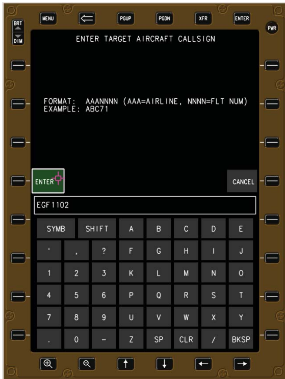
Figure C-17. Manually enter the target aircraft call sign
