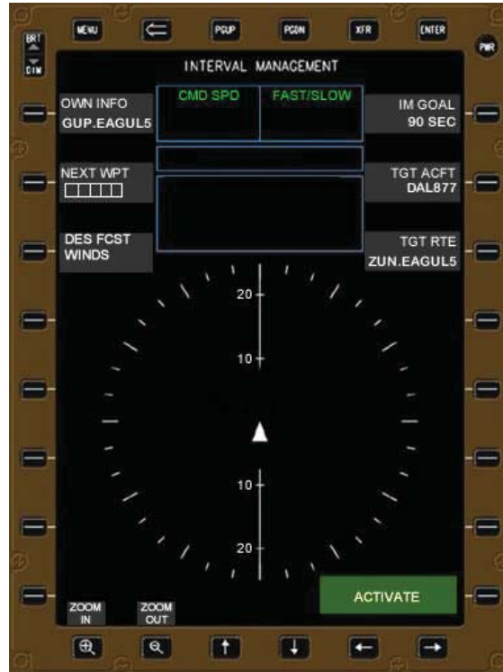
Figure C-21. Activate the IM operation
