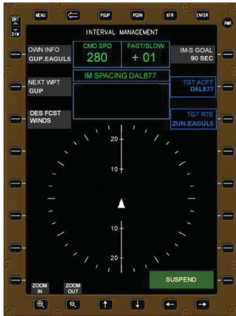
Figure C-30. Cancel IM spacing by first suspending FIM operations
