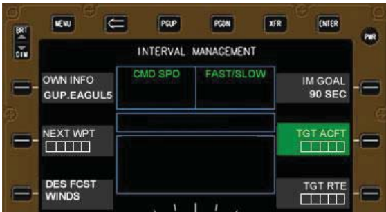
Figure C-14. Load the target aircraft call sign
