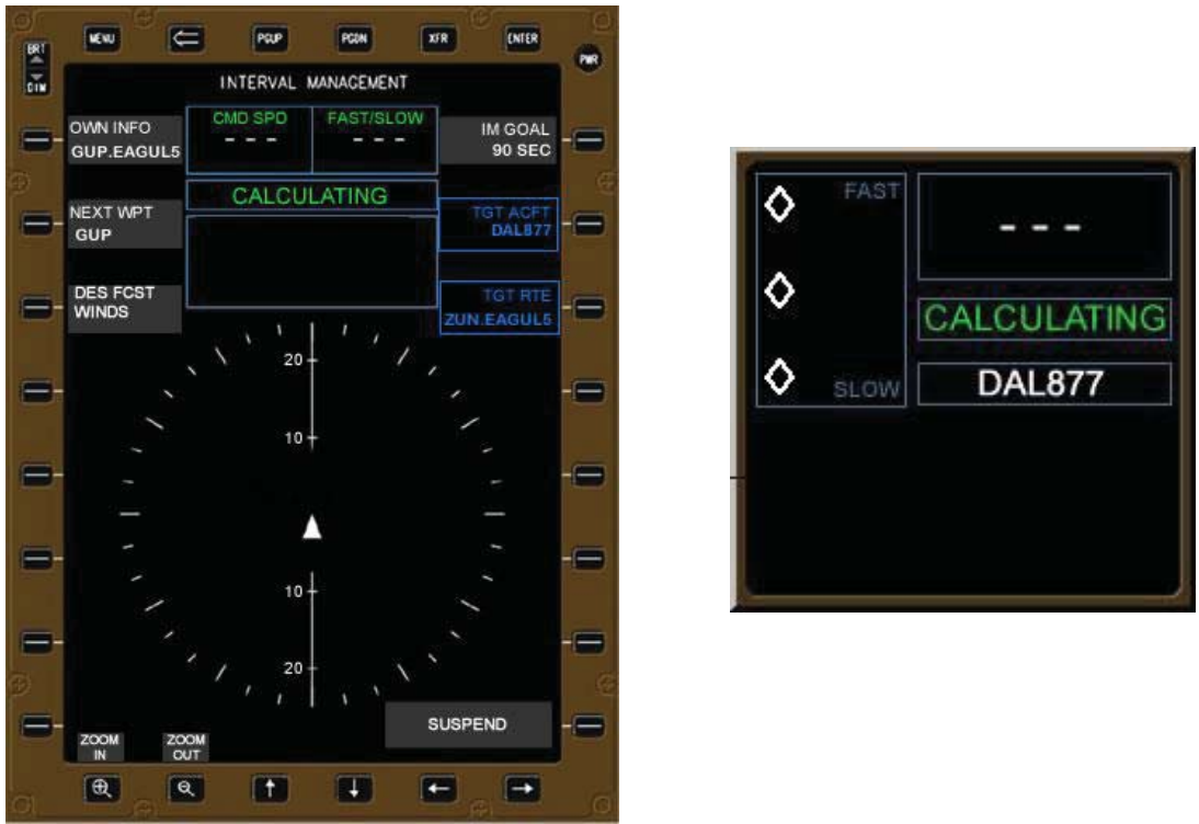
Figure C-22. Calculating initial speed command
