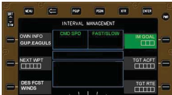
Figure C-12. Load the assigned spacing goal
