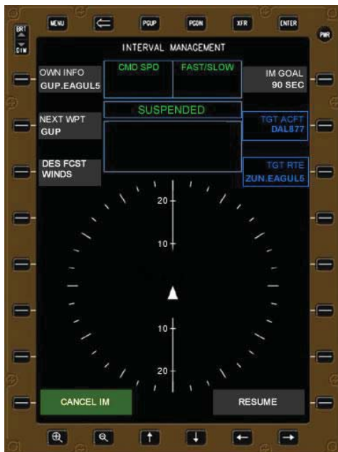
Figure C-30. Cancel IM spacing by first suspending FIM operations
