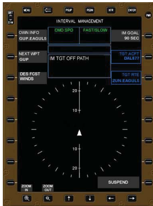
Figure C-29. Unable spacing due to target off path
