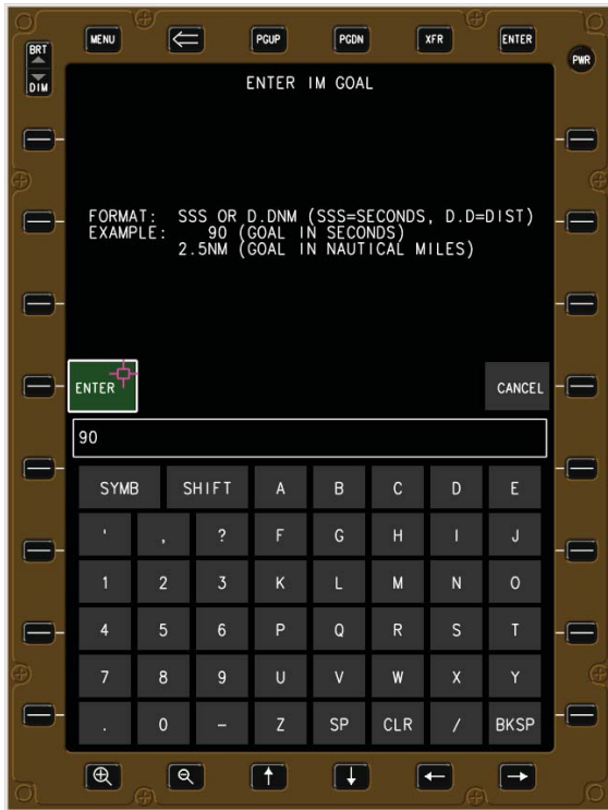
Figure C-13. Enter the assigned spacing goal
