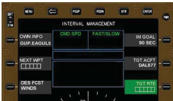
Figure C-18. Load the target aircraft route information
