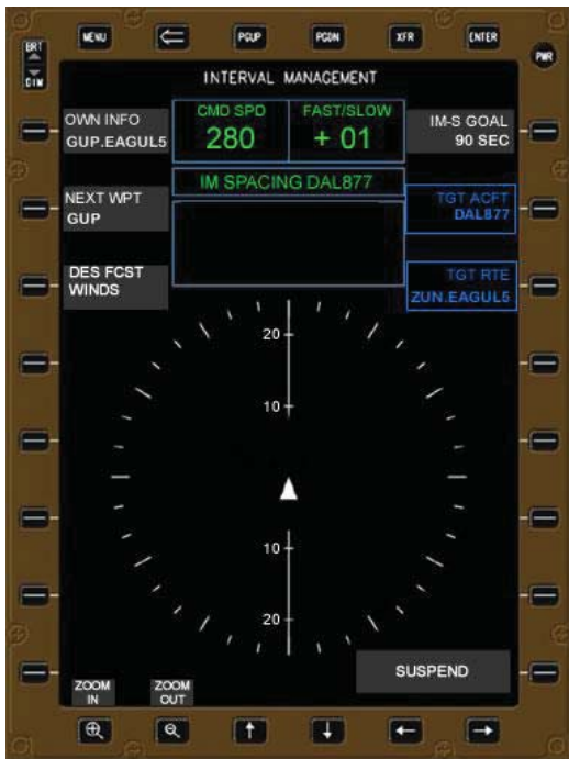
Figure C-28. Interval Management Main Page with IM spacing resumed
