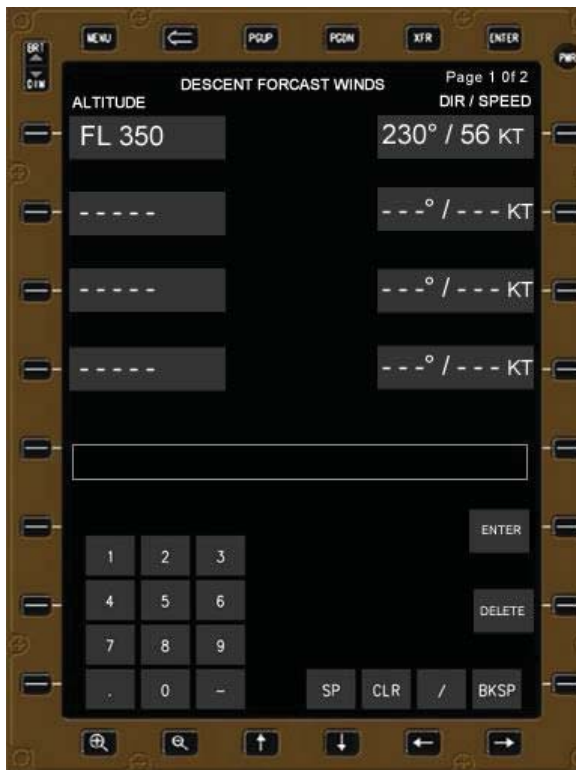
Figure C-10. Load the wind direction, speed, and altitudes
