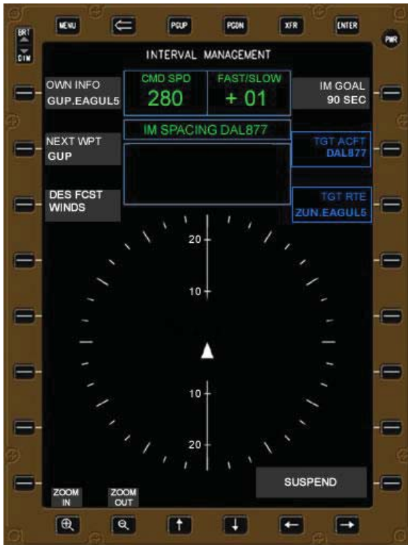
Figure C-24. Amend the assigned spacing goal
