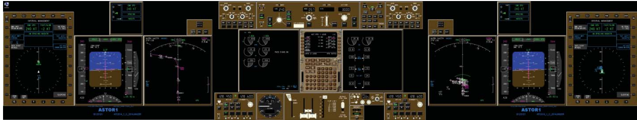
Figure 11. Dual-crew ASTOR desktop simulator displays
