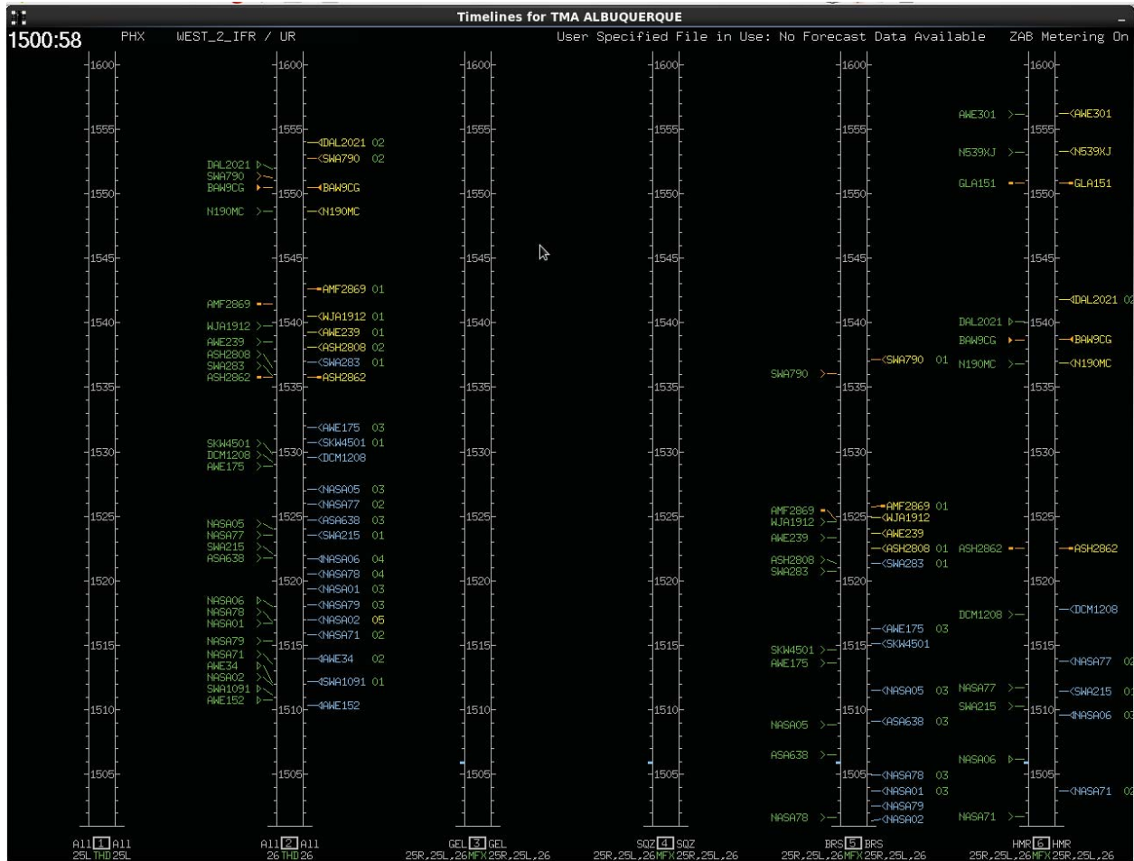
Figure 4. Traffic Management Advisor with Terminal Metering display
