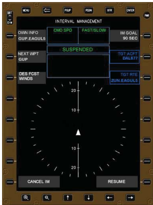
Figure C-26. Interval Management Main Page with IM spacing suspended
