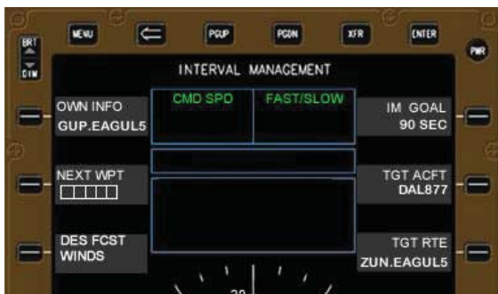
Figure C-20 Interval Management Main Page with assigned spacing goal, target aircraft call sign, and target aircraft route information
