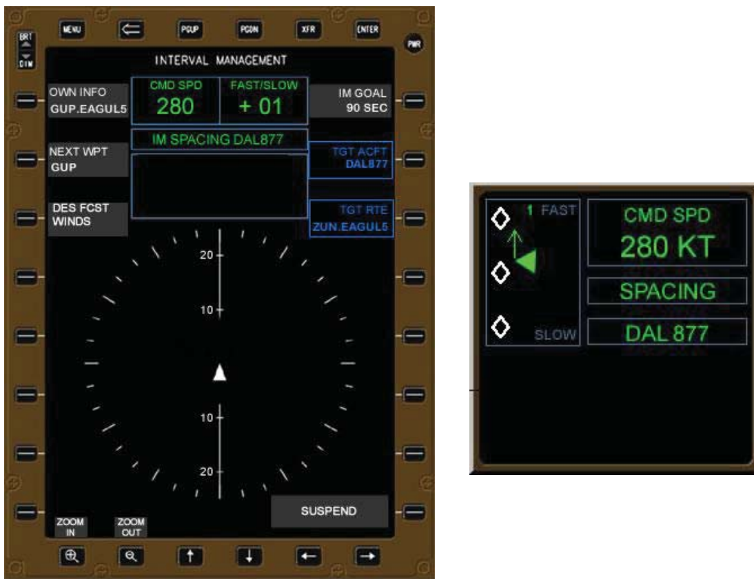
Figure C-23. Information displayed on the EFB and CGD while performing FIM operations
