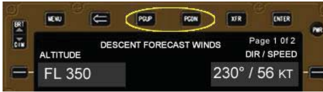
Figure C-11. Switch between pages on the EFB
