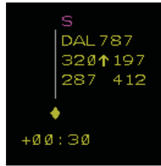
Aircraft has reported paired spacing with target aircraft
