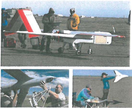
Figure 7. UAS used during MIZOPEX included SIERRA (top), ScanEagle (bottom left) and DataHawk (bottom right)
