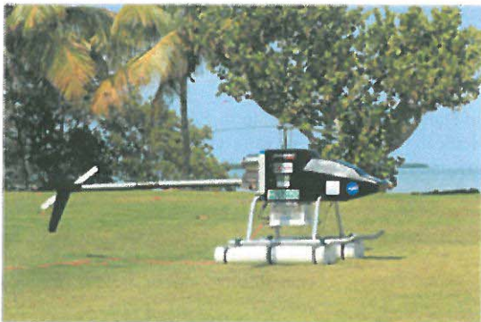
Figure 4. Vision-II UAS carrying NovaSol hyperspectral imager
