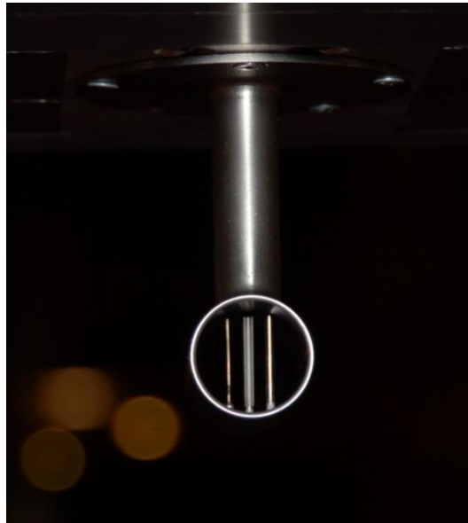
Figure 14.—The Multi-wire liquid water content instrument mounted in the icing tunnel.
