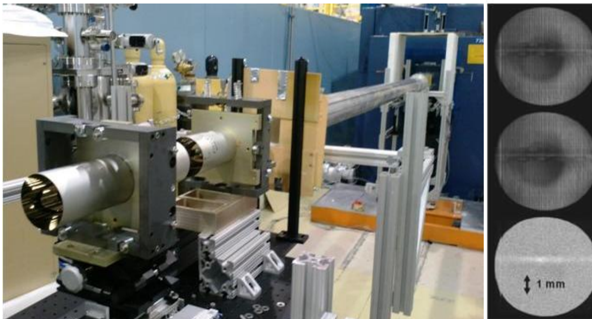
Figure 10. A neutron beam line at NIST (Left) for demonstration of cold-neutron imaging for potential use in a permanent beam line for diverse research applications. One such applied-research use is to measure the accumulation of water on a fuel-cell electrode (Right).
