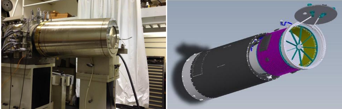
Figure 6. Micro-X ENR x-ray optics, showing fabrication of the first mandrel (Left) and a schematic of the optical bench (Right).
