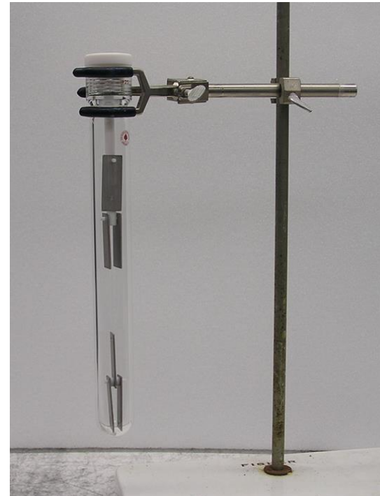
Coupons set in High Pressure Rated Glass Tube.
