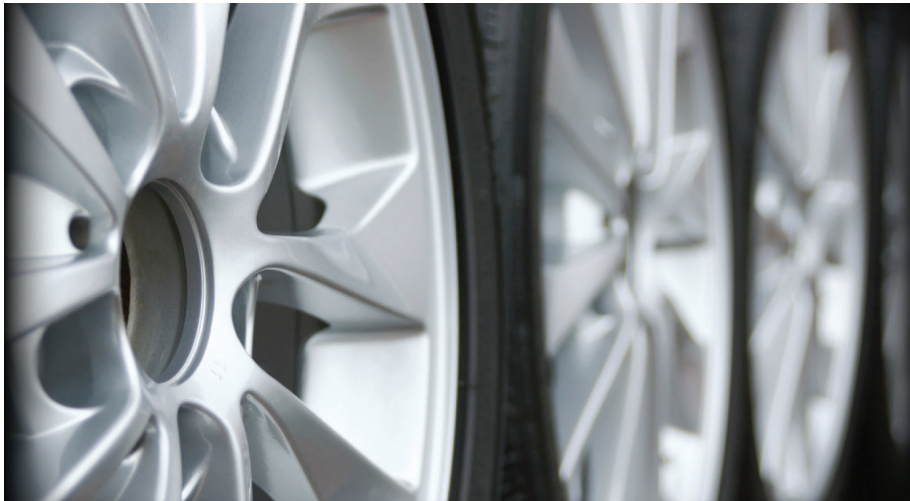
FIGURE – NASA-427 may enable cast aluminum wheels with high strength, low weight, and less costly processing.
