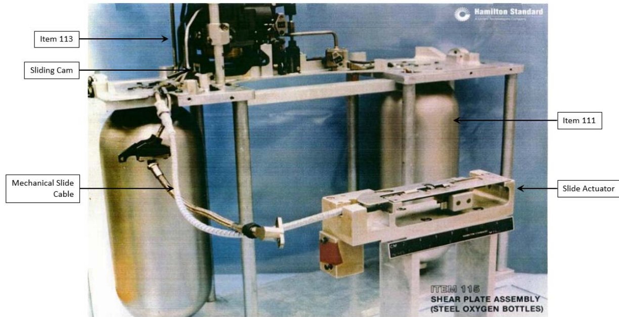
Figure 11 - EMU Shearplate Photo
