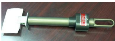
Modifying the EVA Brush Kit handle to accept a commercially available sterile swab will result in a cost-effective EVA-compatible swab tool
