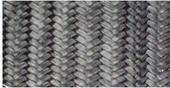
Figure 3. T650-35, 6K Triaxial Braid [0/+60/-60]
