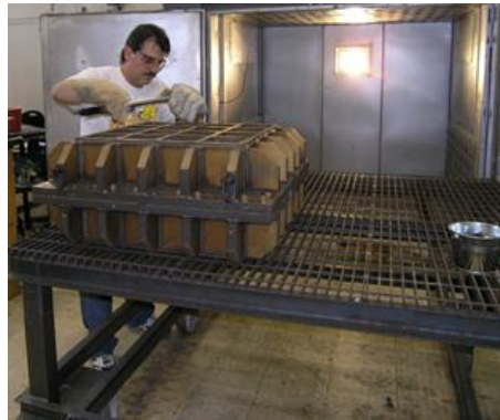
Figure 2. High temperature RTM tool used for 61 cm x 61 cm (2' x 2' ) panel fabrication
