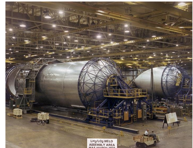
Space Shuttle External Tank major weld area. 1977
