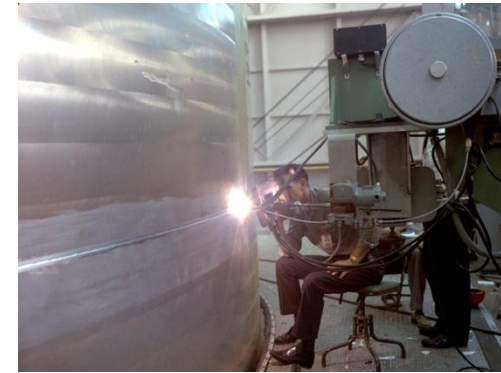
Above: Closeout welding operation of the liquid oxygen tank for the Saturn V SA-501 vehicle for the Apollo 4 mission. 1965
