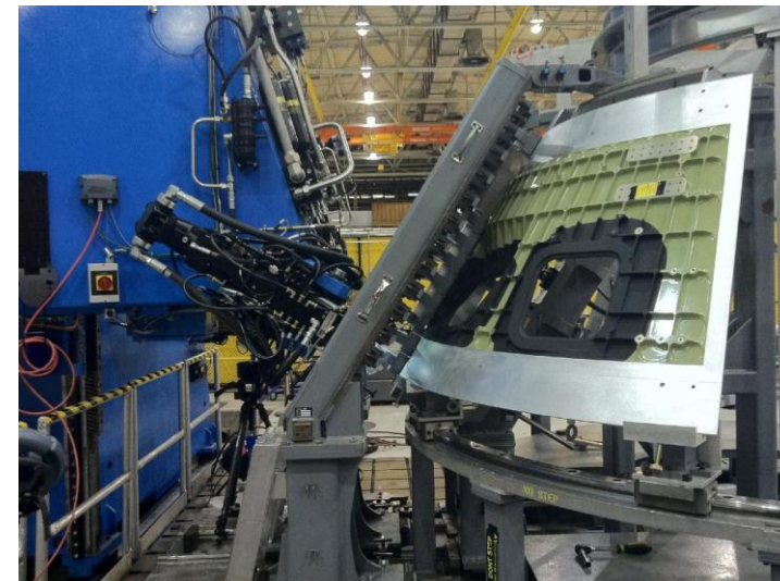
Welding of the Orion capsule at MAF. [2]
