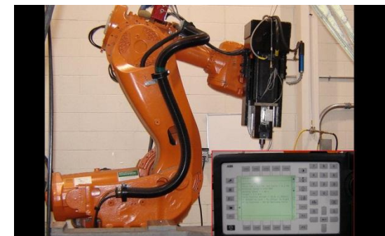
Articulated FSW Robot [14] 20
