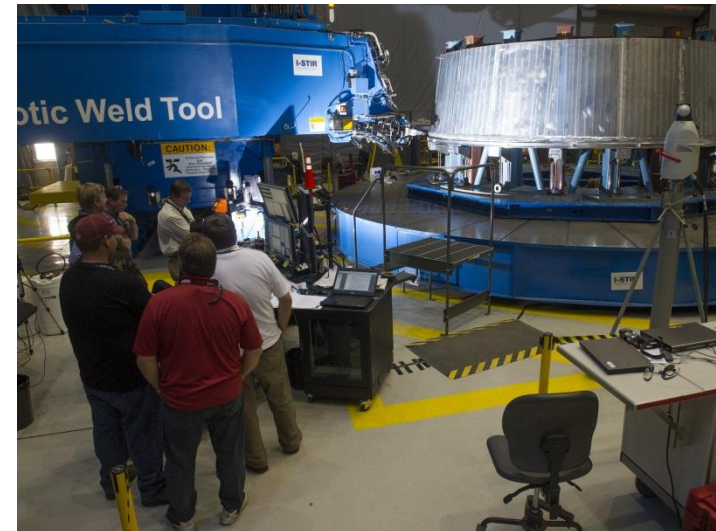
Welding of the SLS spacecraft adaptor at MSFC. Nov 2012 [1]
