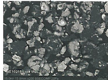
Scale up and down-selections of commercial source NASA HfO_2 -Si EBC Bond Coating Powders
