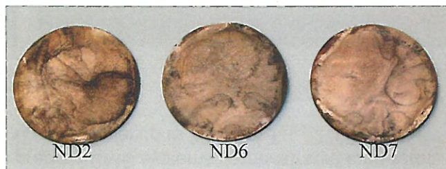
High pressure burner rig tested new ND series Hybrid EBC systems coated on 2" diameter Gen II Prepreg SiC/SiC CMCs
