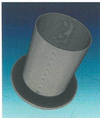
NASA CT scans showing some defective regions of a 0/90 layup element
