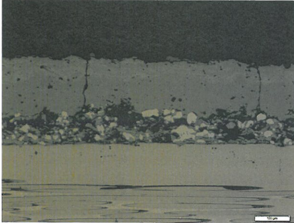
EBCs on Gen II CMC after 1000 hr fatigue testing
