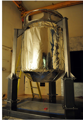
LH2 Active Cooling – Thermal Test (RBO) and Acoustic Test (VATA)
