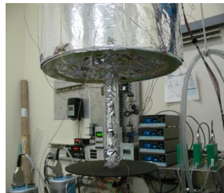
(MLI) Penetration Heat Leak Study
