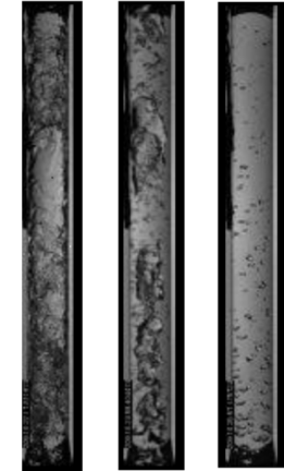
Sight Glass during Line Chilldown
