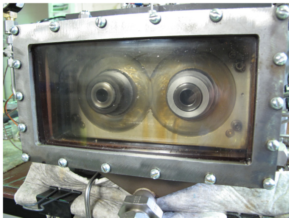
Figure 2. Top exit shrouds with normal lubrication conditions.
