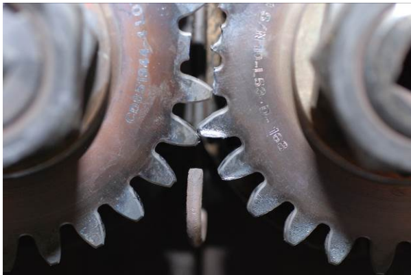
Figure 20. Close up of instrumented and unshrouded gears post-test.
