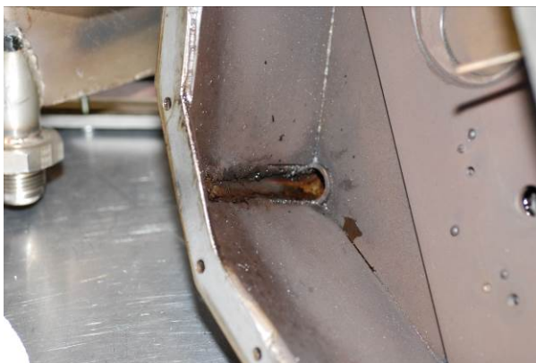
Figure 21. Close up of gearbox cover post-test for unshrouded gear test.
