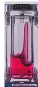
45° vane angle in microgravity.
