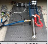
Eccentric to Concentric (E:C) Overload Assist Device—ZIN Technologies Device combines the benefits of a pas-
