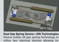
increased resistive loads, two cable outputs, and increased resolution at low loads.
