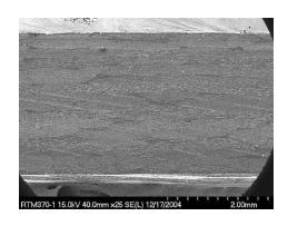
RTM370 Made by RTM Void content = ~1% Resin content = 44-47%
