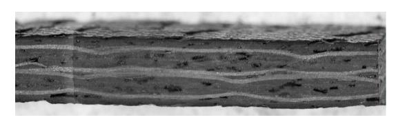
SEM of RTM370 made by VARTM Void content = ~6.5% after postcured at 650°F/8 h Resin vs fiber content =47-50% vs 53-50%
