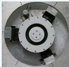
4 kW HIVHAC Thruster & Hall Propulsion System
