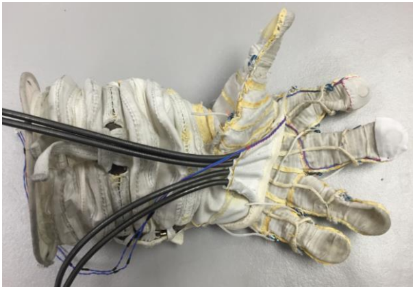
Fig. 7. Early prototype for RoboGlove integration with a space suit glove
