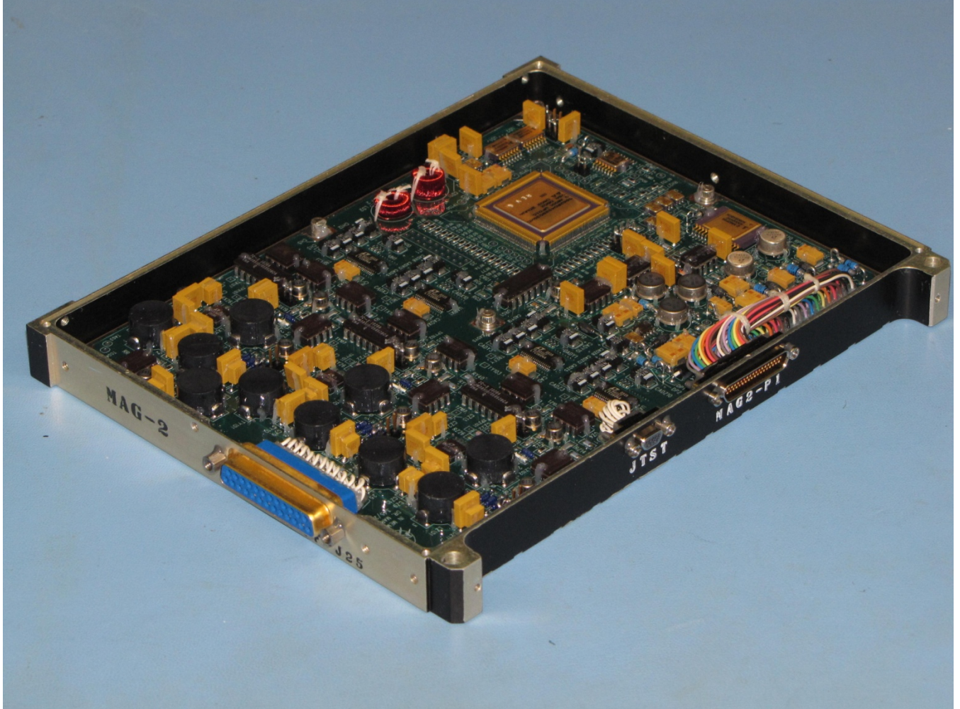
1214 1215 1216 1217 Figure 13: Magnetometer analog and digital board (one of two identical assemblies) in its 1218 shielded frame, top cover removed for viewing. The analog portion is to the left, where the 1219 sensor cable connector J25 resides, and the digital portion is to the right. The FPGA is the 1220 large square device on the upper right. 1221 1222 1223
