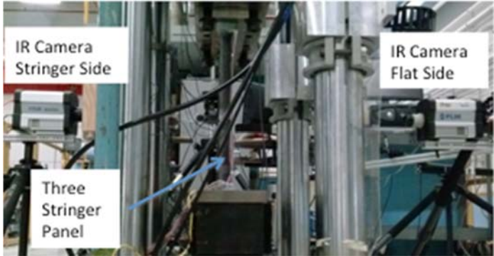
Figure 2. Three-stringer panel setup for passive thermography inspection of both flat and stringer sides.
