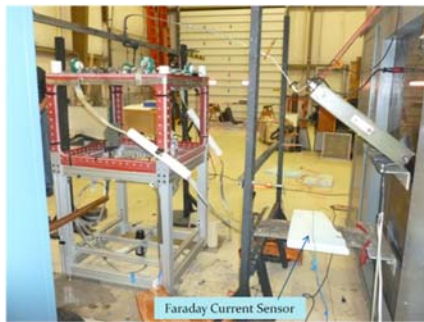
Figure 7. A high-current measurement setup and data for 100 kA and 200 kA on a current return plate.
