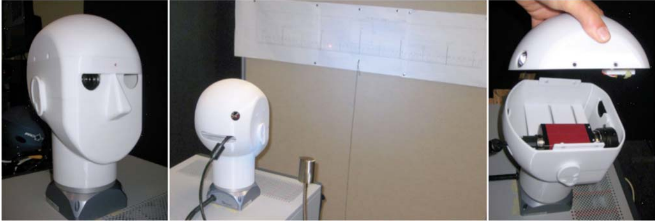
Figure 8. HeLMR System (Head, Camera, Rotary Stage, Stage Controller, DC Light Source).
