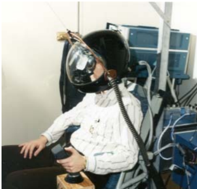
Figure 1. Monochrome, binocular HMD circa 1988, 9 pounds.
