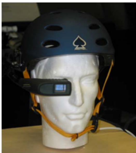
Figure 9. Full color, monocular HWD circa 2007, 2 pounds. Outside-in laser head tracking.
