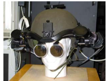
Figure 3. Full color, binocular prototype HMD by Microvision circa 2003, 10 pounds.
