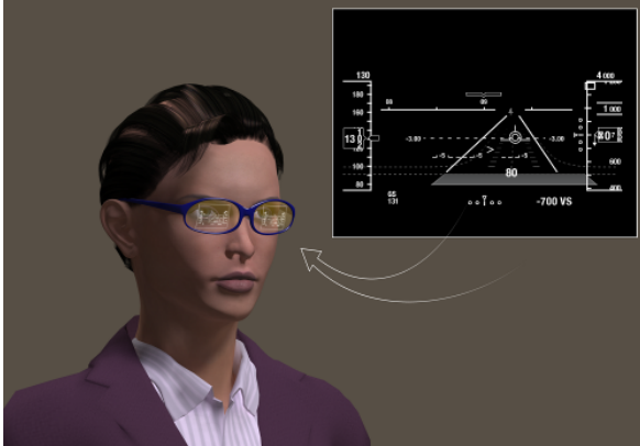
Figure 4. Concept picture of a light-weight, sunglasses form factor HWD for commercial aviation use.
