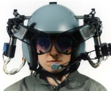
Figure 2. Monochrome, binocular HMD circa 1991, 6.5 pounds.
