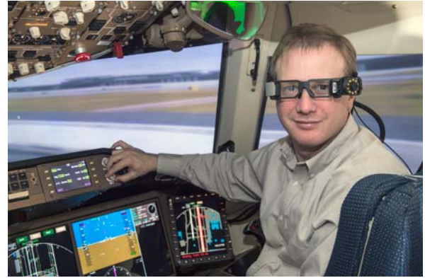
Figure 5. Lumus DK-32 display glasses coupled with a prototype inside-out head tracker made by Thales Visionix.
