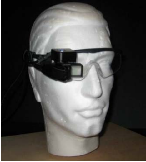
Figure 6. Monochrome, monocular HWD circa 2010, 4 ounces.
